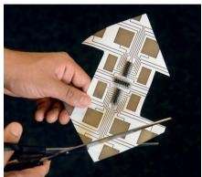
Snipped: A pair of scissors can bring this sensor into nearly any shape and size.
