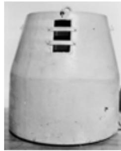
Erich Regener (below) gave his name to this steel barrel, or "Tonne," designed to protect atmospheric measuring instruments.
