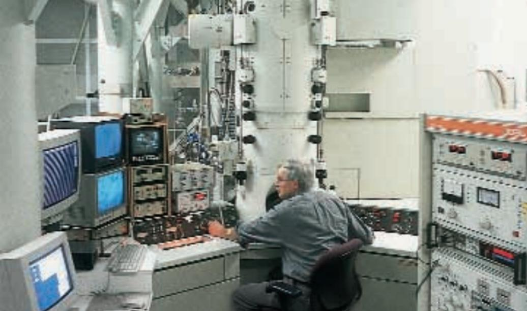
*The Atomic Resolution Microscope (ARM) set up at the Max-Planck-Institute for Metals Research in Stuttgart is one of the three maximum performance microscopes in the world and the only one located outside Japan. By operating this maximum resolution transmission microscope (1,250 kilovolts) atomic structures – the position of atoms at interfaces or contact surfaces, for example – become visible.*
