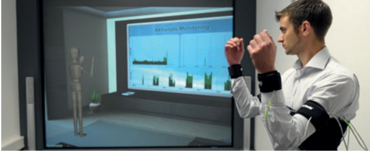
Sensor technology allows body movements to be transferred to digital models in real time.
