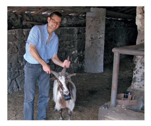
Grabbing the goat by the horns: For his field trial, Martin Wikelski fitted a few animals with transmitters that he had specially produced for the study. At the front of the collar is a battery pack that supplies power for many months. The GPS logger and the electronics are located on top, where reception and transmission are strongest.
