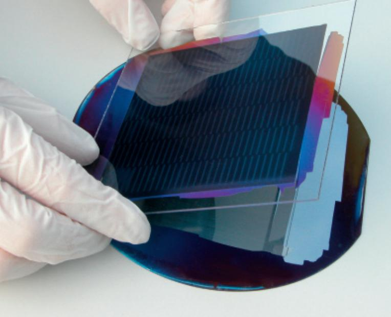
Peelable solar cell: A member of the ISH team presses an adhesive-coated piece of glass onto the extremely thin crystalline silicon layer and peels it off the wafer.
