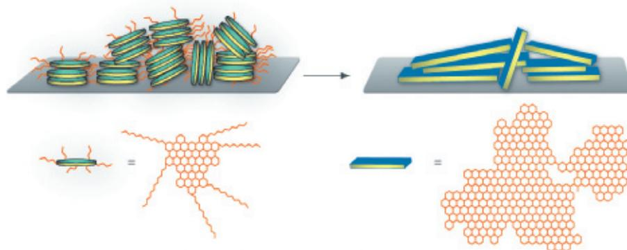
Carbon puzzle: Under the influence of heat, little slabs of graphite with hydrocarbon chains attached (left), combine to form larger graphite layers (right).
