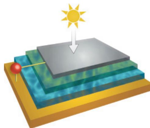
Solar cells, a matter of layers: The photo-voltaically active materials, such as dyestuffs and titanium dioxide, lie between two electrodes – the top one must be transparent.
