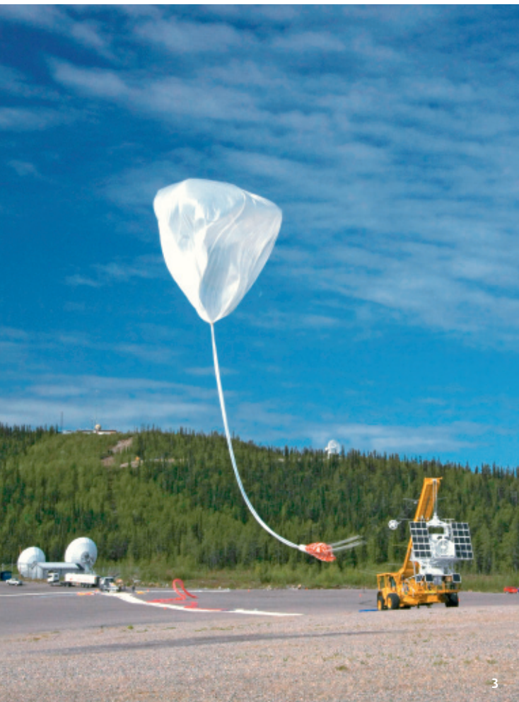
Final preparations for the solar observatory Sunrise , whose main mirror is one meter in diameter [photos 1 and 2]. Then, on June 8, things get serious: While the observatory hangs from the mobile crane, the helium balloon slowly straightens up [3]. Shortly afterwards, the balloon pulls Sunrise upward with a jolt [4] – the two-hour journey to the stratosphere has begun [5].
