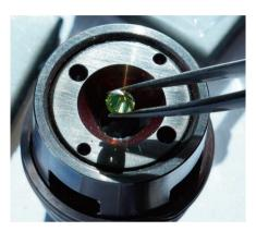
Many states: Diamonds are used to put elements under pressure in a diamond anvil cell
