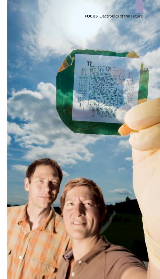
left: The researchers in Stuttgart use an evaporator to deposit organic semiconductors onto overhead transparency film, and also onto banknotes. They deposit the substances onto the substrate through a shadow mask in order to produce the structures of transistors.
