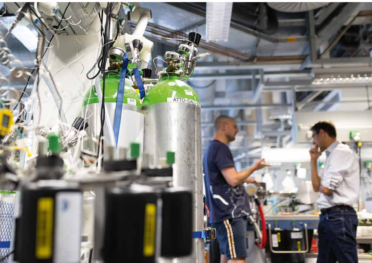
Hot on the trail of greenhouse gases: Heiko Moossen (left) and Sönke Zaehle are researching the increase and decrease of nitrous oxide, as well as carbon dioxide and methane, in the atmosphere, and analyzing their isotope ratios with mass spectrometers for this purpose. The pure substances from gas cylinders serve as a reference here.
