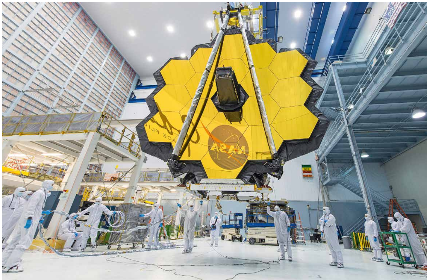
Honeycombs for the heavens: the primary mirror of the James Webb telescope consists of 18 hexagonal beryllium segments and has a diameter of six and a half meters. With it, the observatory surveys the universe in infrared light.
