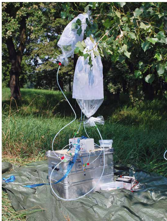
The researchers capture the gaseous odor signals of the leaves in plastic bags and pass them through a filter. They then determine the chemical structure of these volatile substances in the laboratory.
