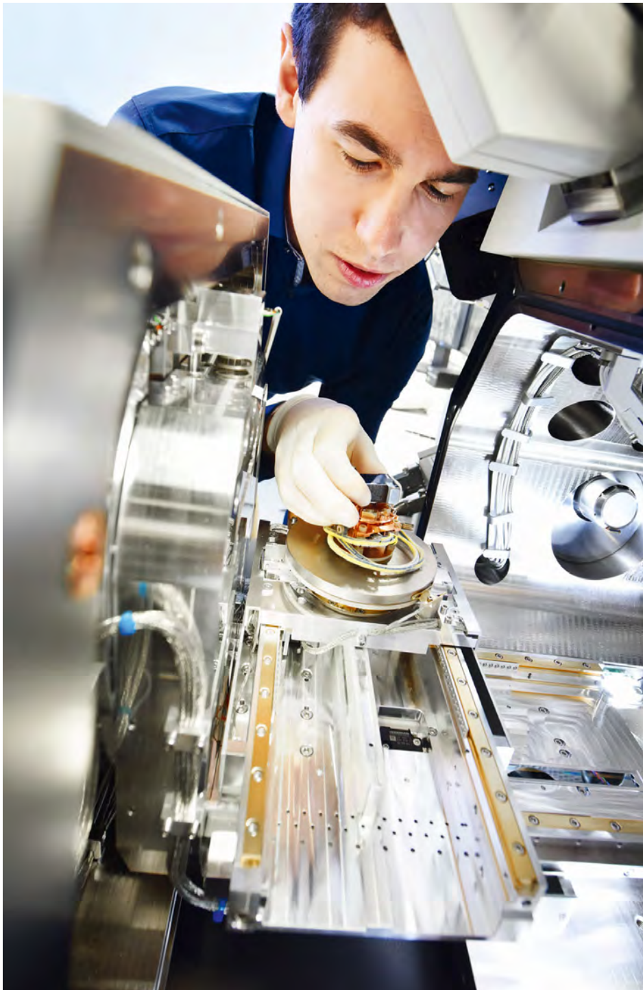
Freshly printed metal: Philipp Kürnsteiner inspects a cube-shaped sample of steel comprised of alternating tough and hard layers. The researcher created the material using a sophisticated method that allowed him to control the 3D printing process.
