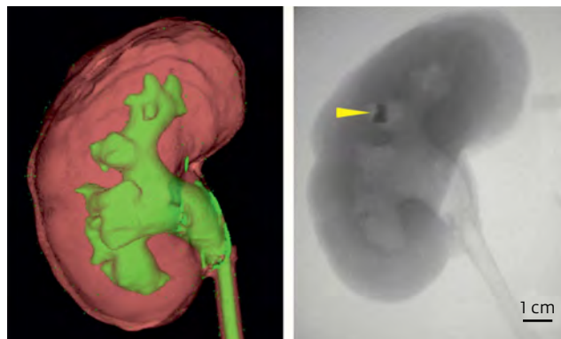
Phantom kidney: on the left a 3D design, on the right an x-ray of a printed organ model in which a tumor has been positioned (arrow).
