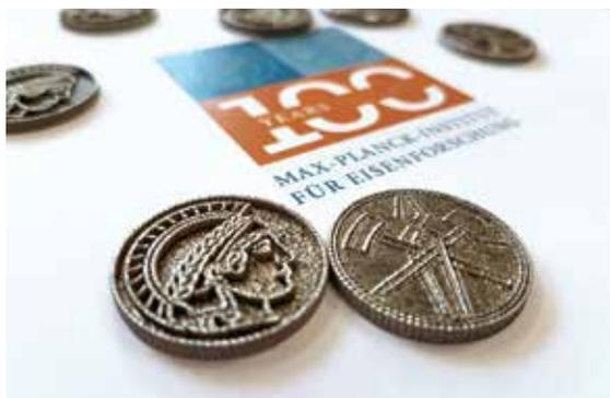
One example of the complexity of components that can be produced by additive manufacturing: the logo of the Max-Planck-Institut für Eisenforschung as a relief on 3D printed coins of stainless steel.
