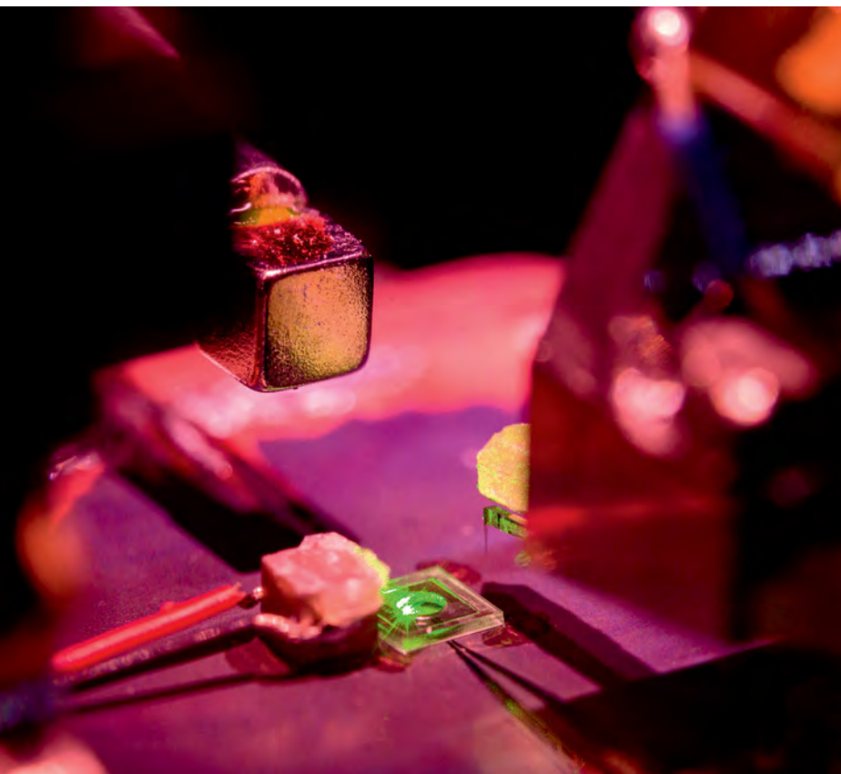
The Stuttgart-based researchers use a diamond to measure the field of a cube-shaped magnet (left). The intensity of the glow from the quantum sensor when irradiated with green laser light depends on the strength of the magnetic field.
