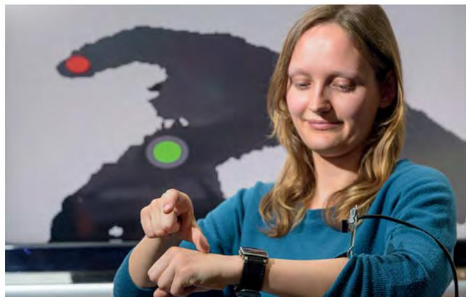
A new type of remote control: WatchSense enables users to control electronic devices, such as smartwatches, with finger movements on and above the back of the hand by tracking the tips of the thumb and index finger.
