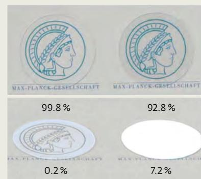
A glass plate on which nanocolumns have been etched (illustrations on the left) reflects just 0.2 percent of light falling on it at an angle of 30 degrees and is transparent to the remaining 99.8 percent. At the same angle of incidence, a plate without the surface nanostructure (illustrations on the right) transmits only 92.8 percent of light, reflecting 7.2 percent.
