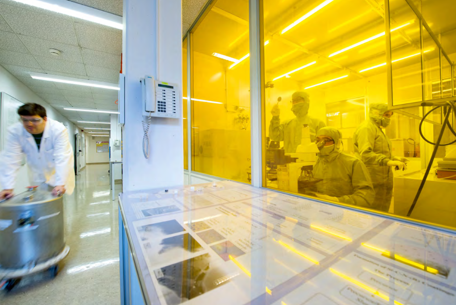
Dust obstructs: In the clean room, the researchers use photolithography to create microstructures, such as the micro-scallop. It is crucial that they avoid even the tiniest impurities in the air.
