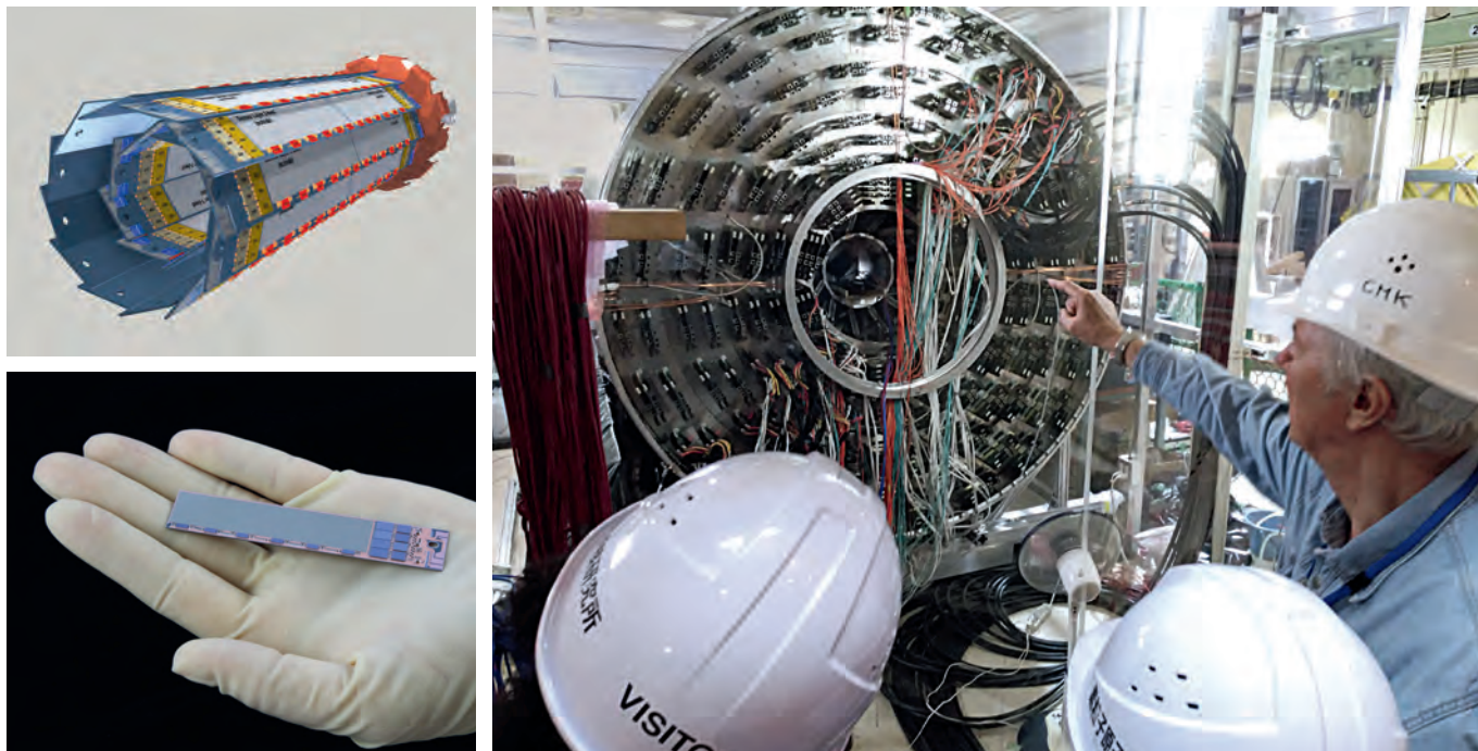
Christian Kiesling (right) and his colleagues assess the progress as the Belle-II detector at SuperKekB is being set up. Kiesling points to an opening that will house the vertex detector, whose task is to determine the exact position of the decay. The heart of this instrument is the dual-layer pixel detector (top left), inside which the decays take place. It is composed of modules whose image sensors each comprise 200,000 pixels (bottom left).
