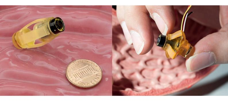
Gastroscopy usually requires patients to swallow an endoscope tube. Although camera-carrying capsules are also suitable for the task, it is still not possible to control them. Scientists at the Max Planck Institute for Intelligent Systems in Stuttgart plan to change all that. And their tiny capsule-shaped robots can do a lot more than merely take snapshots of the stomach's interior.
