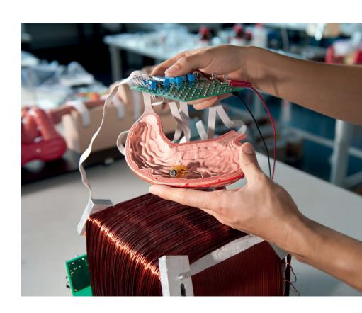
proved successful. Metin Sitti filled the small chamber of the MASCE with micro-grippers and positioned it with the help of a magnetic field on a piece of pig's stomach. When the capsule was compressed in the magnetic field, the micro-grippers fluttered down onto the tissue. When the researchers increased the temperature, the micro-grippers snapped shut.
