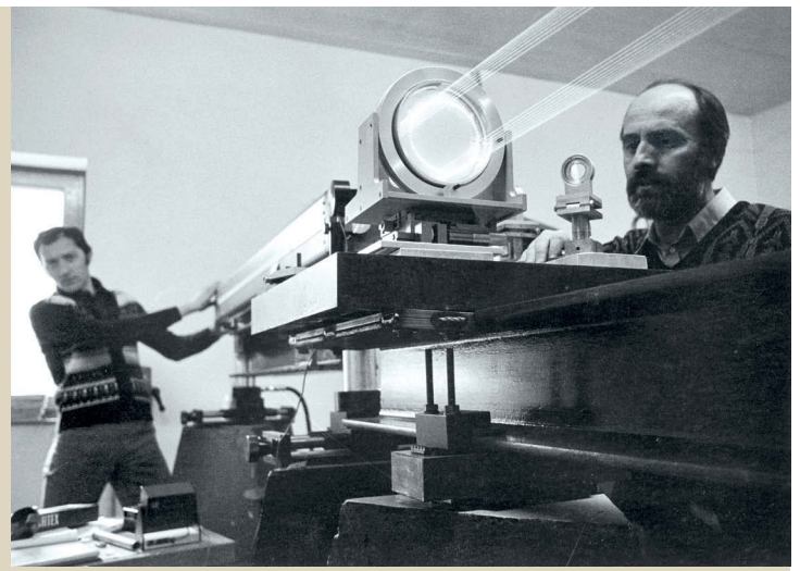
New technology: Lasers form the heart of the second generation of detectors. Here, Walter Winkler (background left) and Karl Maischberger are working on the prototype of such an interferometer in 1977.
