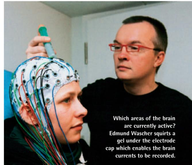
Which areas of the brain are currently active? Edmund Wascher squirts a gel under the electrode cap which enables the brain currents to be recorded.
