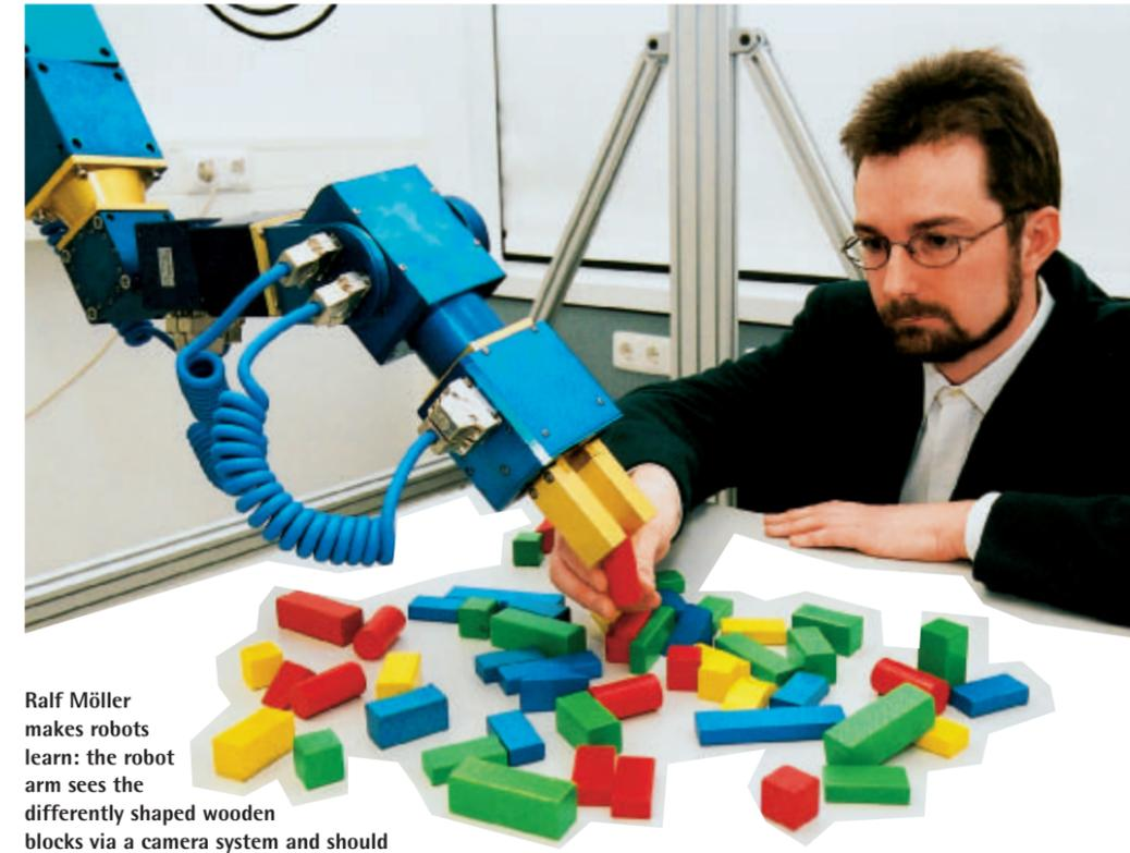
Ralf Möller makes robots learn: the robot arm sees the differently shaped wooden blocks via a camera system and should be able to pick them up properly.
