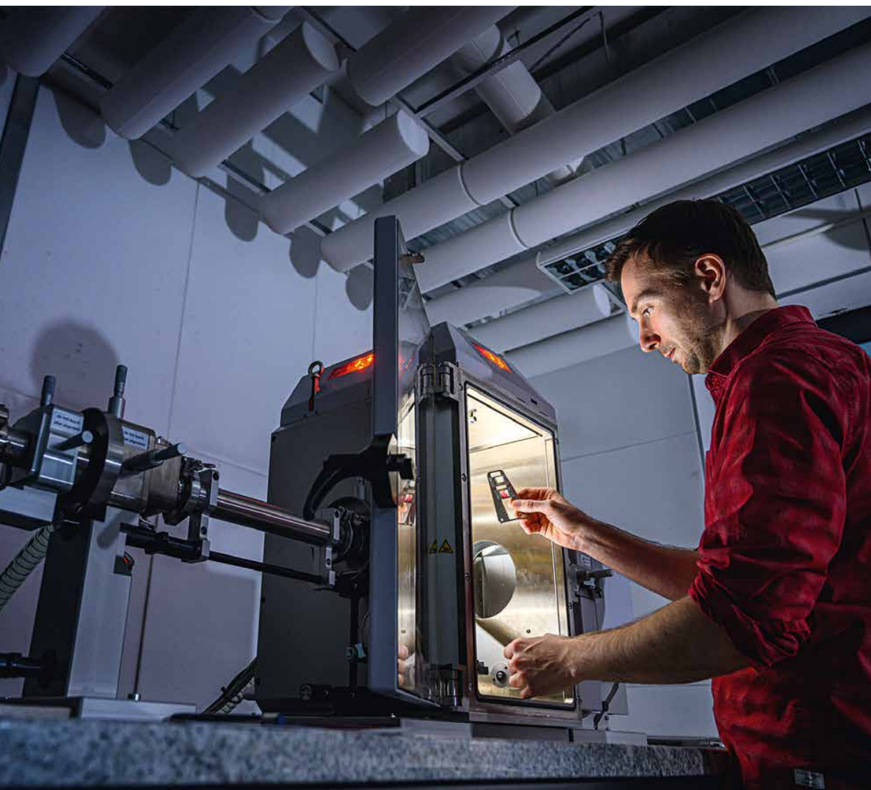
Sample for the “nanostar”: technician Daniel Werner prepares to analyze a sample of bone using small-angle X-ray scattering (SAXS) to determine the size of its mineral particles.
