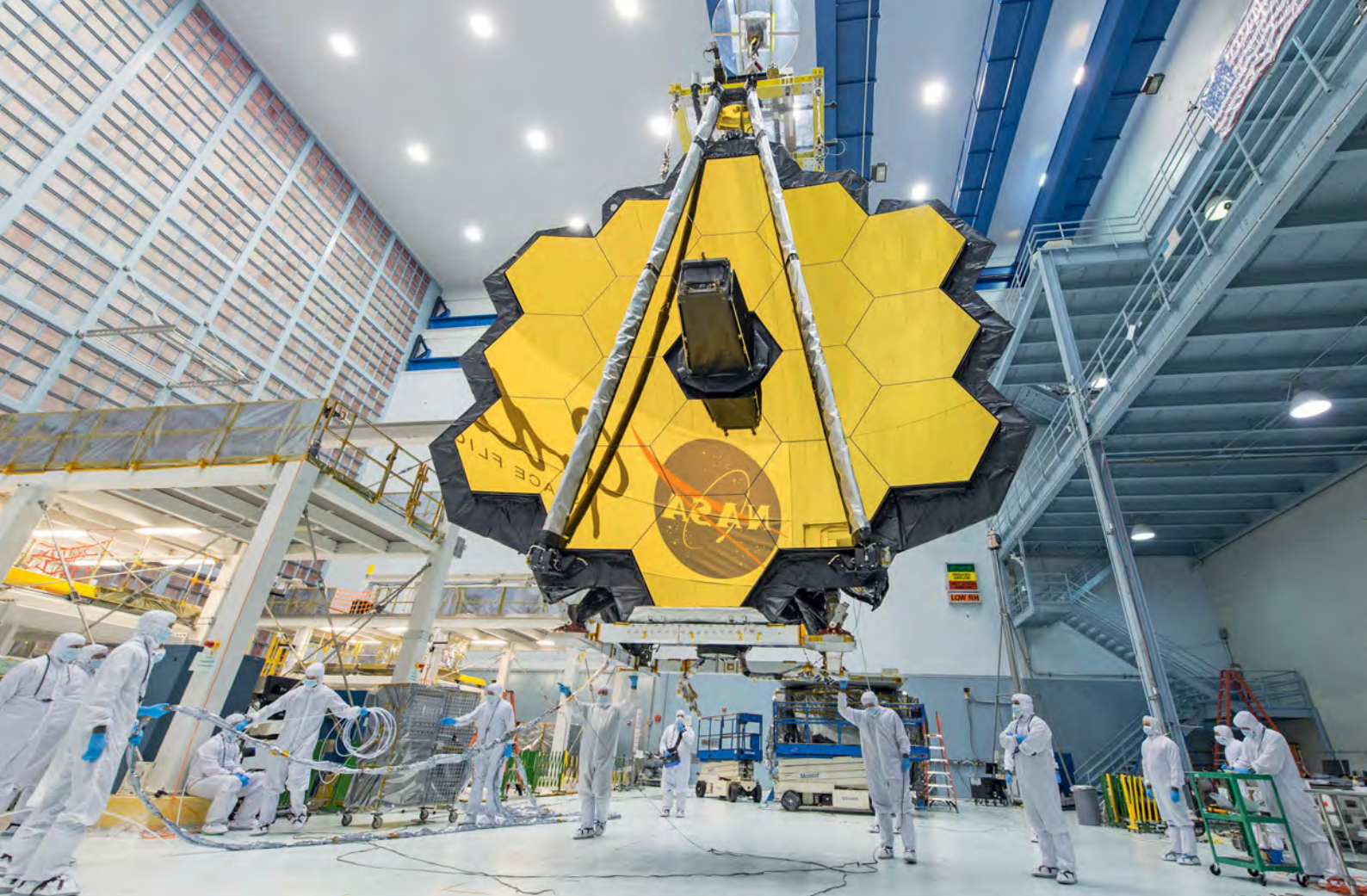
A gigantic compound eye: the gold-sputtered main mirror of the James Webb Space Telescope has a diameter of six and a half meters and is made up of 18 segments. From May 2020, at the earliest, the instrument will scour the heavens and train its sights on distant exoplanets.
