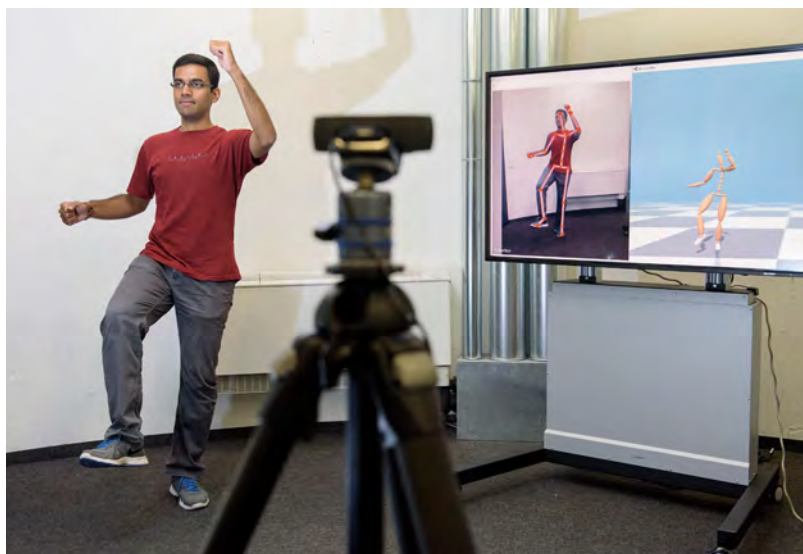
Srinath Sridhar demonstrates how well VNect calculates a three-dimensional model of the researcher's body poses in real-time based on images captured with an inexpensive webcam.
