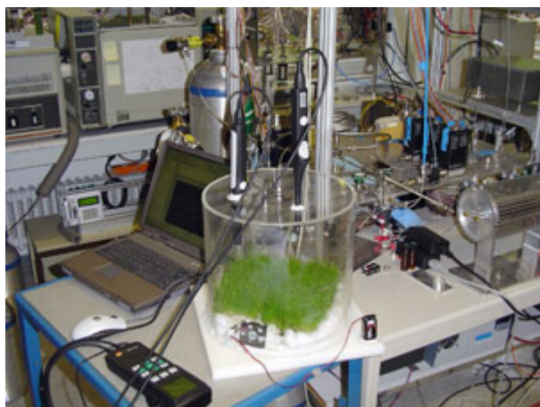
Image 1: A plant chamber used to investigate methane formation in plants -- in this example, in ryegrass ( Lolium perenne ).
