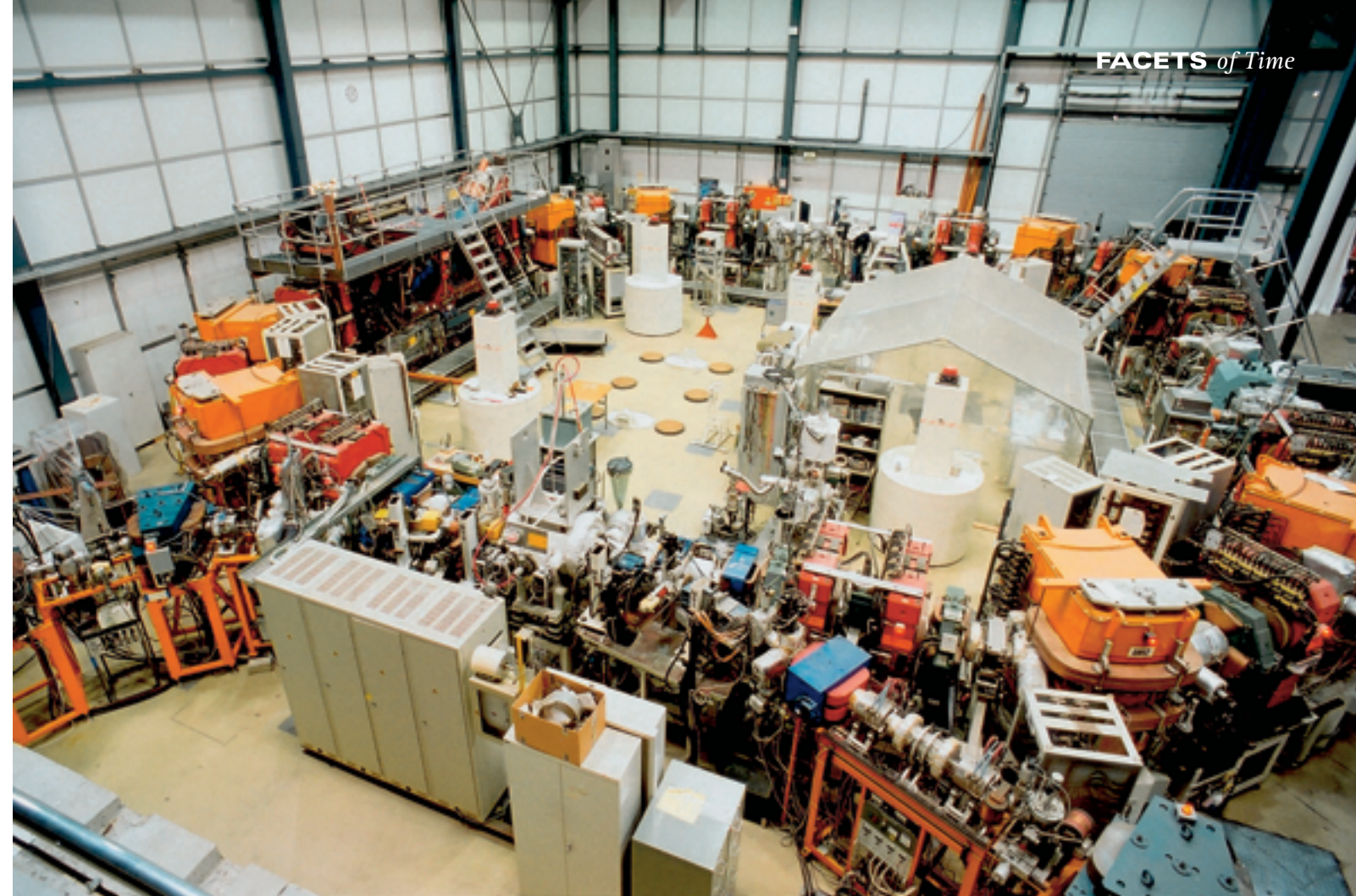
A "racetrack" for particles: In the Test Storage Ring in Heidelberg, lithium ions race at a speed of 19,000 kilometers per second. Researchers use this to measure the effect of time dilation.
