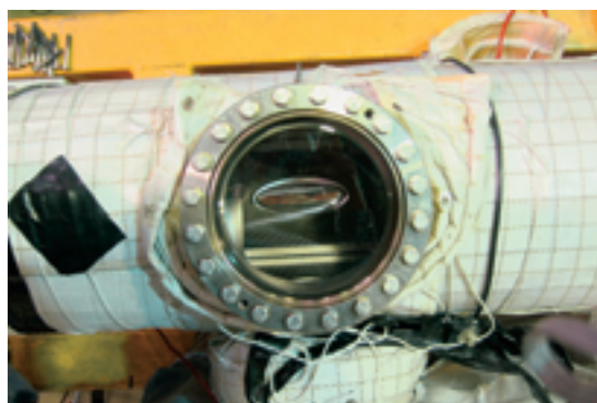
Peering into the pipe: A window in the steel pipe of the Heidelberg storage ring allows the photometer to register the glowing ions.
