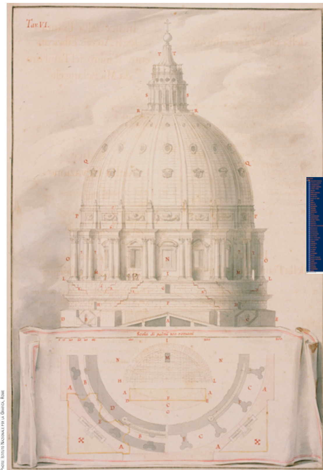
Luigi Vanvitelli: Investigation of the structural condition of the dome of St. Peter's, 1743.
