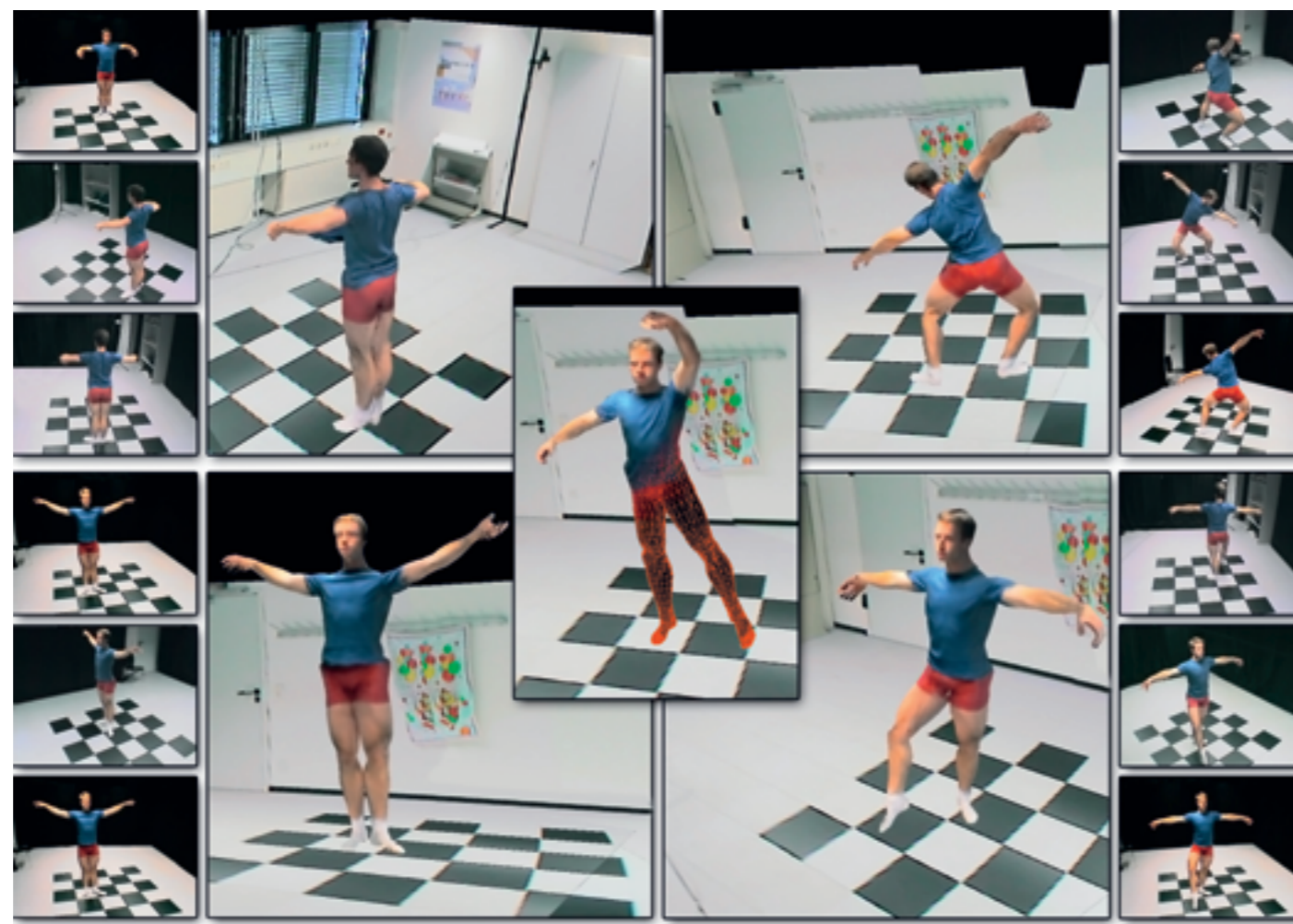
The movements of the dancer are recorded by eight synchronized video cameras, then aligned with a digital human model – temporarily transforming the dancer into a Spiderman of sorts.
