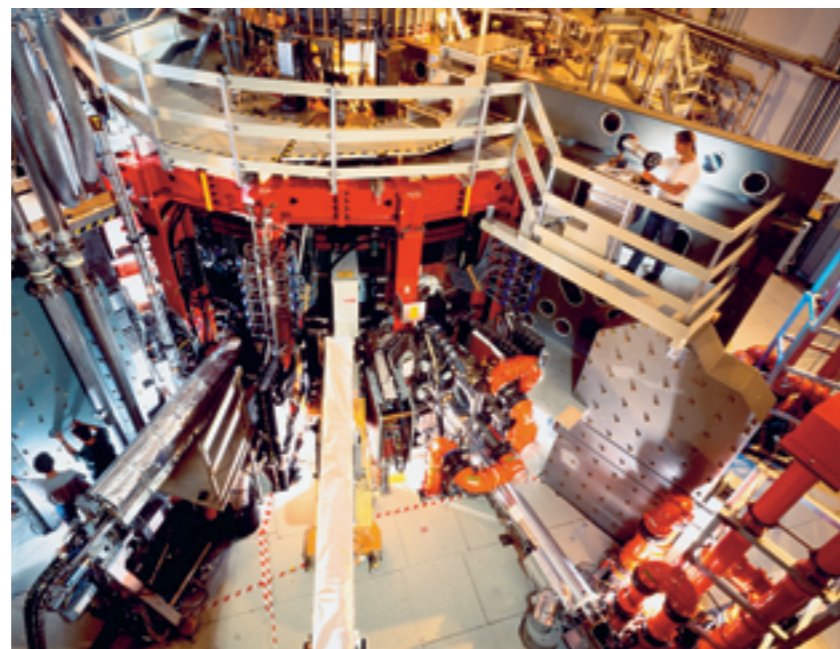
A glimpse into the "oven": The ASDEX Upgrade tokamak is the largest fusion experiment in Germany. At the left of the image is the waveguide for heating the system through the application of radio waves.
