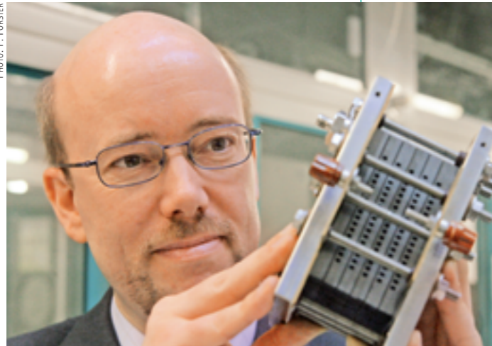
Kai Sundmacher, Spokesman for the joint ProBio project and Director at the Max Planck Institute for the Dynamics of Complex Technical Systems, with a stack of PEM fuel cells that are powered by hydrogen.
