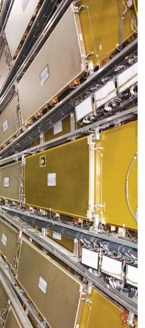
left One section of the world machine: The ATLAS detector in the Large Hadron Collider of the European research center CERN is, like the CMS experiment, used in the search for the Higgs boson. ATLAS is enormous: it measures 45 meters in length, 25 meters in height, and weighs 7,000 tons - as much as the Eiffel Tower.
