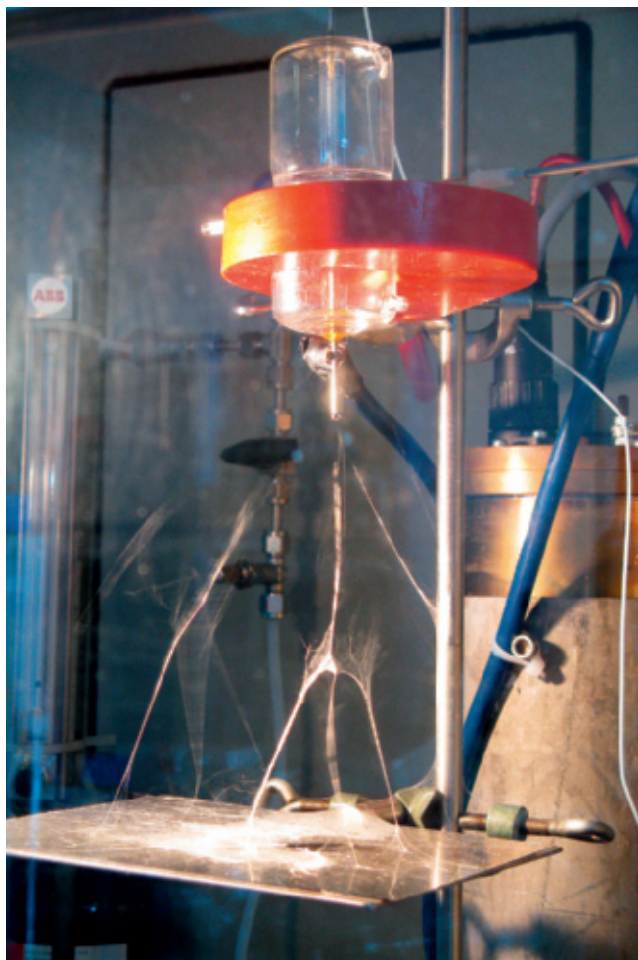
Spinning in the lab: Filaments of an organic material are pulled from the electrode (right). The researchers in Stuttgart use them to produce carbon-tin anodes for lithium batteries that – unlike pure tin – are not destroyed in the electrochemical processes.
