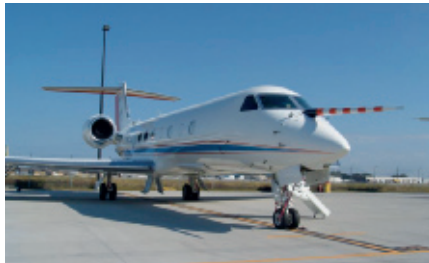
HALO will open up new perspectives for researchers studying the atmosphere. The nose-mounted measuring probe is clearly visible in the photo.
