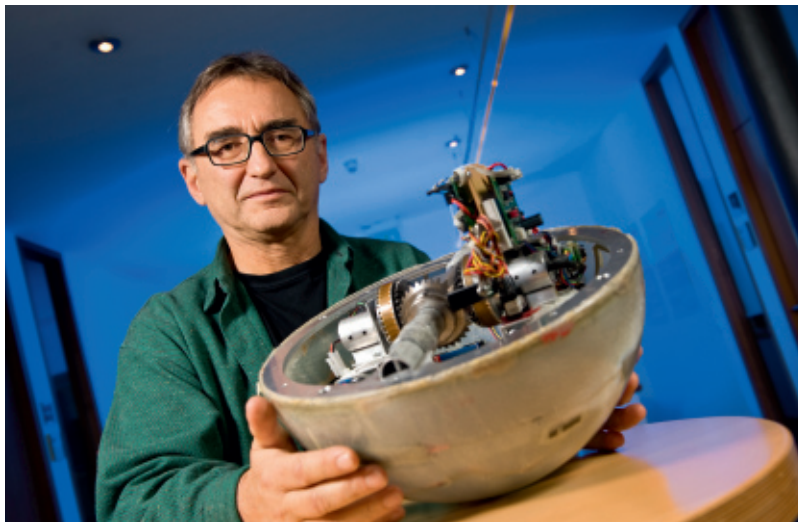
A ball is supposed to learn how to roll: This sphere robot was designed by Leipzig artist Julius Popp. Electric motors push weights inside it to kick it off. Thanks to the brain developed by Ralf Der and Nihat Ay, it can inch its way forward to increasingly complex movement patterns.
