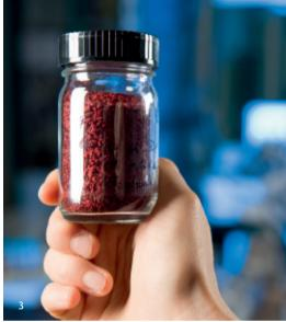
The researchers heat each sample to 800 degrees Celsius in one of the lab furnaces and then test it with a carefully mixed gas. "Right now we are taking particular care to ensure that the materials are stable and can be used for a lengthy period," says Rihko-Struckmann. The powders should be able to withstand a thousand gas and steam cycles.
