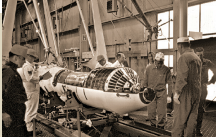
German-American collaboration: Engineers integrate AZUR on a US Scout launcher.
