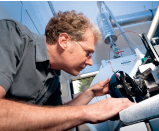
Thorsten Dittmar opens the injection unit of the mass spectrometer. From the syringe at the right edge of the photo, the probe penetrates through the red sheathed capillary into the injection source.
