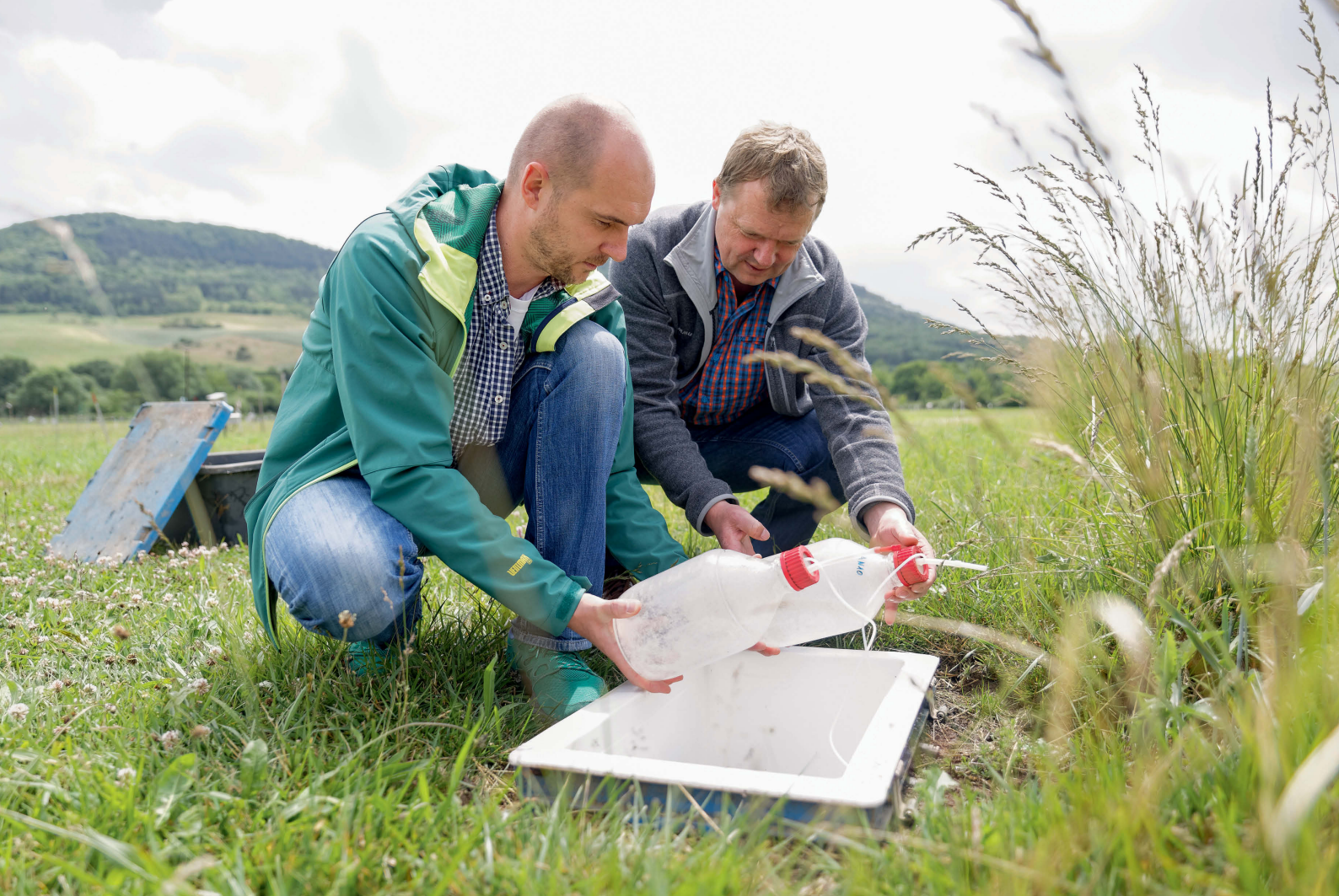
Markus Lange (left) and Gerd Gleixner analyze the organic substances that are contained in the soil water and that reveal much about the processes at work in an ecosystem. The water collects in bottles in which a vacuum prevails. The containers stand in a tub that has been sunk into the ground.
