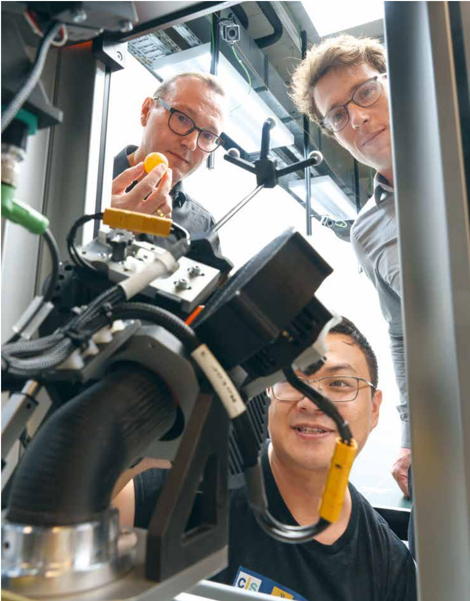
Know your opponent: The table tennis robot on whose control Jörg Stückler, Hao Ma and Michael Mühlebach (from left) are working plays against a ball machine. A model of this machine helps it to hit the fired balls.
