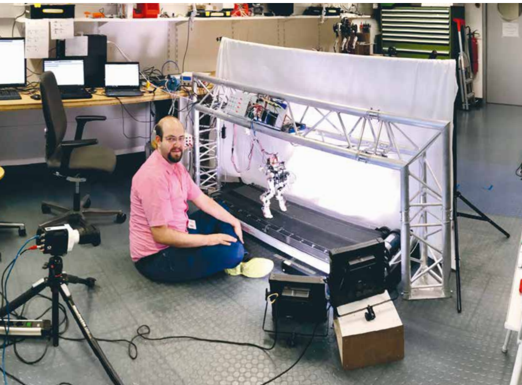
Playground for techies: in his doctoral thesis, Alborz Aghamaleki Sarvestani made BirdBot run and analyzed its gait in experiments on a treadmill. For example, he used a high-speed camera (image center) to shoot slow-motion videos of the robot.
