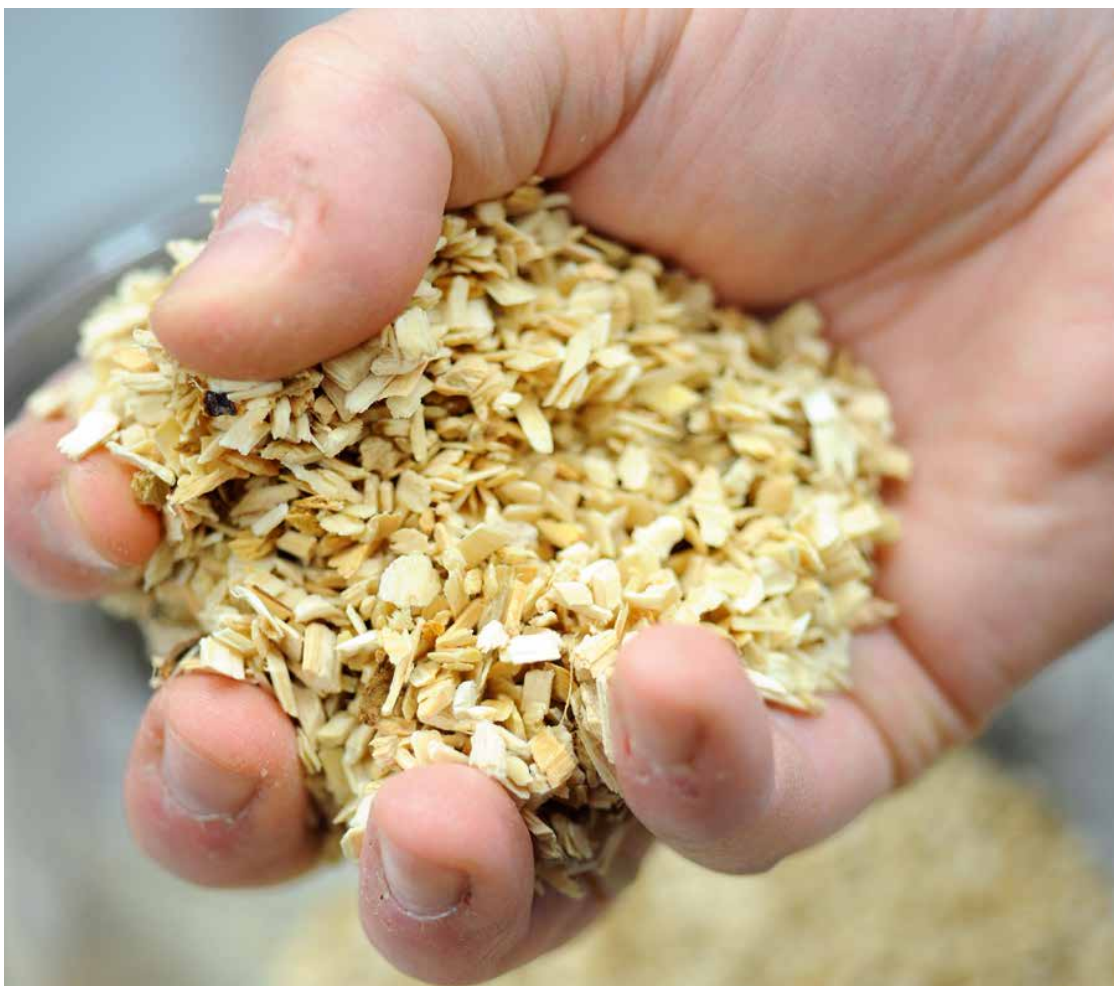
Sawdust as a raw material: wood mainly consists of lignocellulose, from which both biofuel and raw materials for the chemical industry can be derived.
